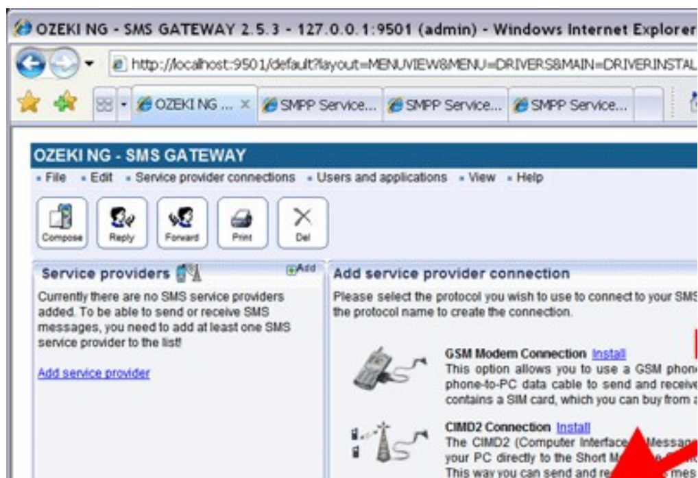
Figure 7 - Install an SMPP service provider connection
