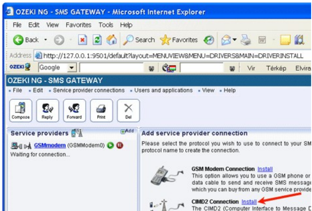
Figure 1 - Starting to install the CIMD2 connection
