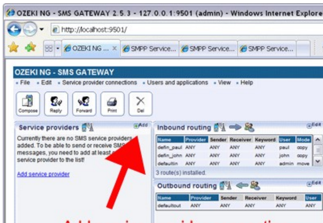
Figure 7 - Click add to start the service provider connection installation procedure
