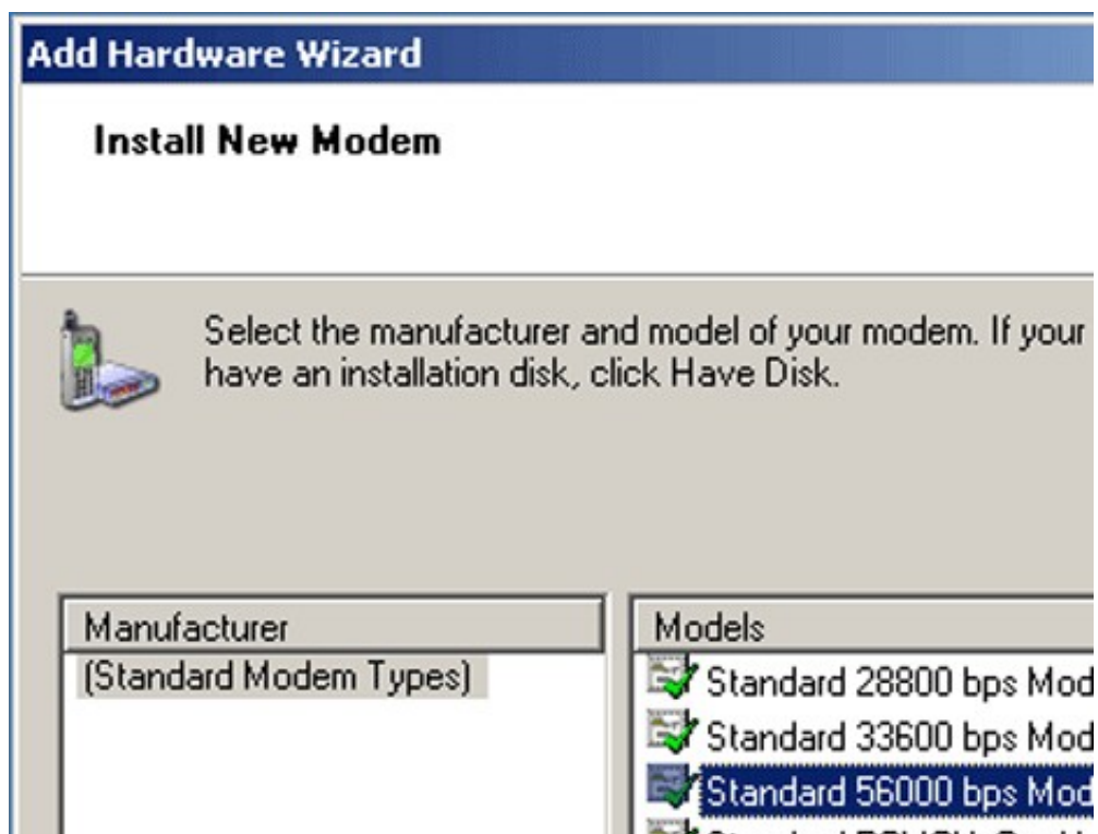
Figure 11 - Selecting the modem driver
